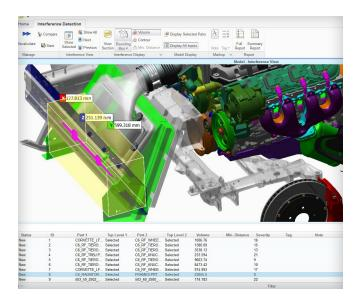
Detect and analyze clash issues with the optional Creo View Interference Analysis module.
