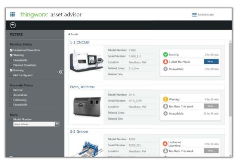
In a single pane of glass, ThingWorx Asset Advisor provides visibility to all the asset on the floor, the asset's current status, generate alerts based on predefined values and can detect irregular operation conditions using anomaly detection.
