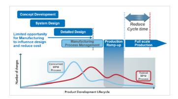
Working concurrently allows Manufacturing to reduce production cycle times, which in turn reduces manufacturing costs
